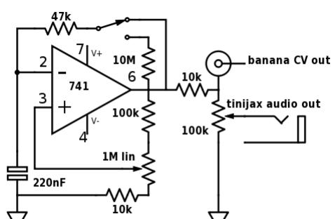
These frequencies may vary depending on the 741, you want to test various values and find the ranges you like. Thanks to a slide switch mounted near the PCB's edge, audio or LFO range can be switched easily. On batch 9 a perboard is available behind the sliders too.
