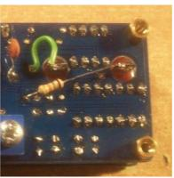
The 100k trimmer is optional and will reduce the pulser trig out voltage for use with external devices needing a trigger signal lower than +15V (eurorack uses +5V gates and triggers). You want to bypass it if not needed and connect the banana socket directly to the trimmer's pin 1. The cable can be replaced with a 1N4148 diode (line to the socket) to protect the output from reverse patching.
