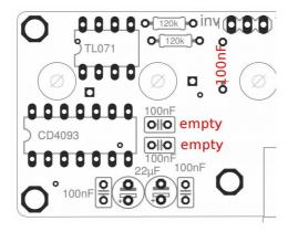
Do not socket the TL071/TL081/LM741, the IC socket corner would upset the banana socket placement. Or snip the socket's corner.
