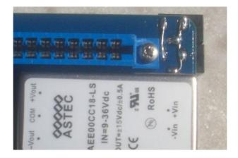
If the optional PSU is not used, bridge the "208 supply" pads to the right to power the Hub's +/-15V rails with the 208's ones, with headers + jumpers or solder components legs.
