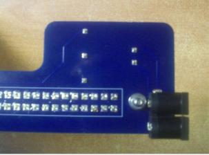
Bridge the 2 tip pads together and the 4 other ones too. This will strenghten the sockets mounting, improve the connection between both sockets and do a proper -Vin connection (the PCB trace connects the -Vin to the socket's switched pad only, this will be fixed on the next batch).
