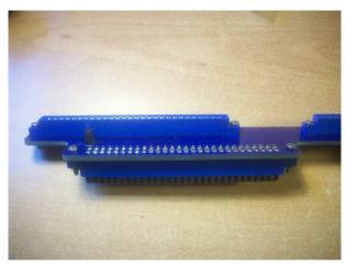
4. If the envelope or pulser bleeds into the LPG1 when the Hub is inserted, add a 33nF capacitor to the back of the left edge connector between contacts 2 and 22 of the bottom row.
