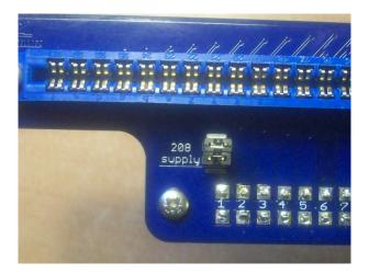
It is still possible to use the 208 supply with the Artesyn AEE00CC18-LS block installed to the Hub as long as it's not powered with an external DC supply.
